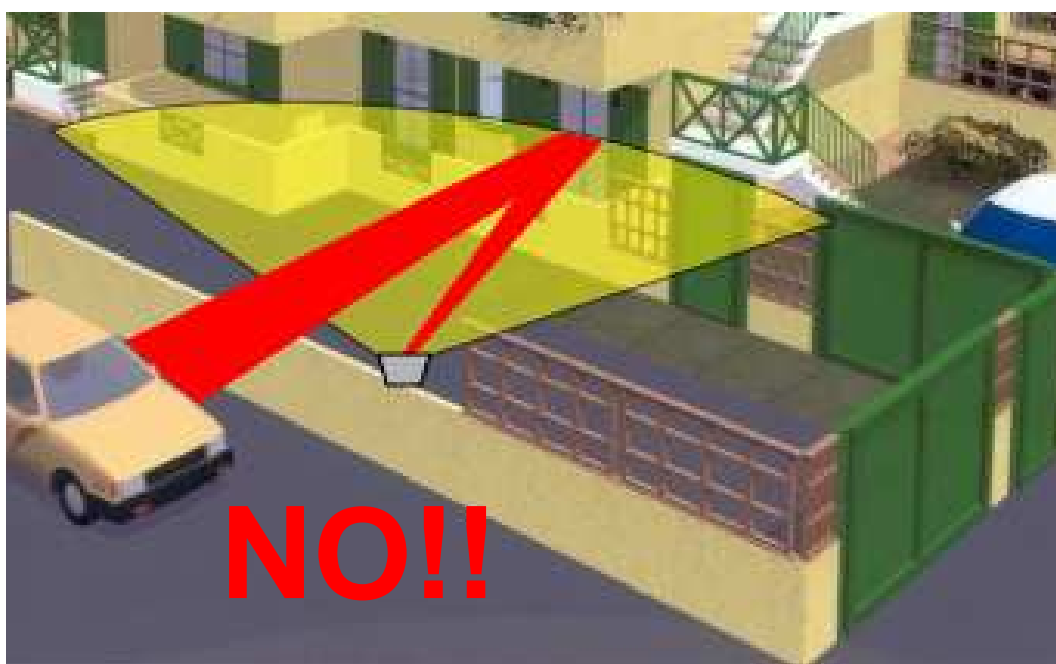
Fig. 4 - Avoid to have beams toward reflecting surfaces.
